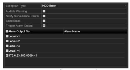
Figure 12-27 Configure HDD Error Alarm
