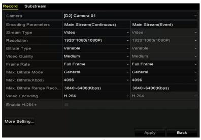
Figure 5-3 Recording Parameters
