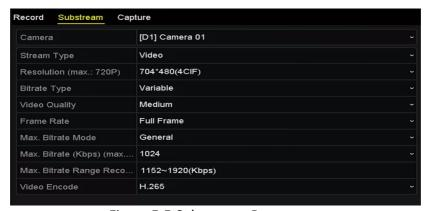
Figure 5-5 Sub-stream Parameters
