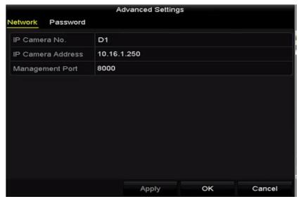
Figure 2-32 Network Configuration of the Camera
