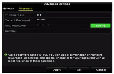
Figure 2-33 Password Configuration of the Camera
