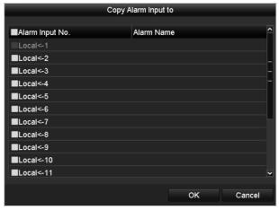
Figure 8-8 Copy Settings of Alarm Input
