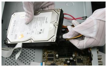
Figure 2-8 Connect Power Cable
