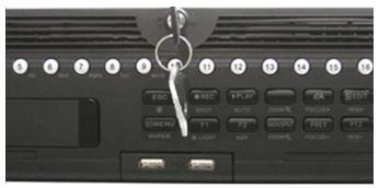
Figure 2-2 Insert Panel Key
