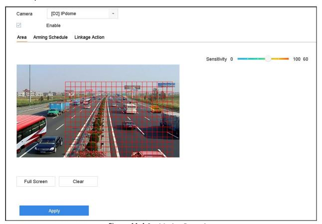
Figure 11-4 Set Motion Detection
