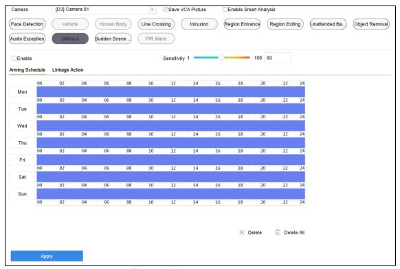
Figure 12-11 Defocus Detection
