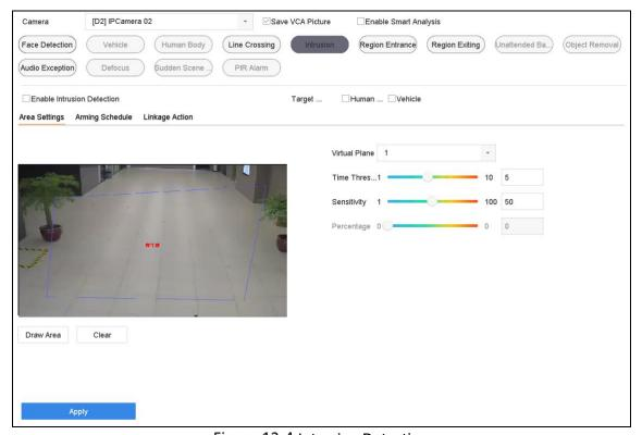
Figure 12-4 Intrusion Detection
