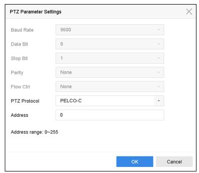
Figure 6-2 PTZ Parameters Settings
