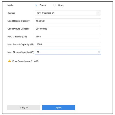
Figure 7-7 Storage Mode-HDD Quota
