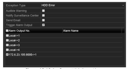
Figure 10-10 Configure HDD Error Alarm
